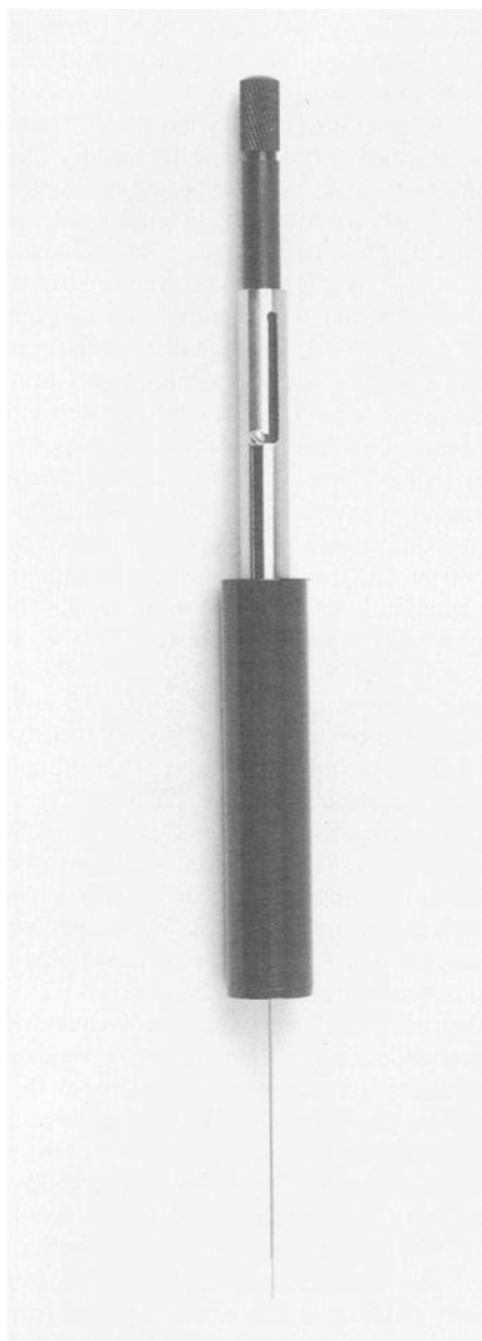
FIG. 1—Photograph of the SPME fiber and assembly used in this work.
